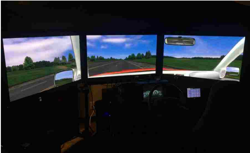
Figure 3.1 miniSim Fixed-Base Driving Simulator
